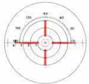
Model:LM-25 Internal Reading System Target:Crossline and Corona
